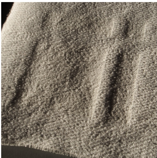
GS: Schlingenzwirn / retors bouclé Nm 3 (2940 m/kg) MS: NeB 12/2 (10 000 m/kg)
